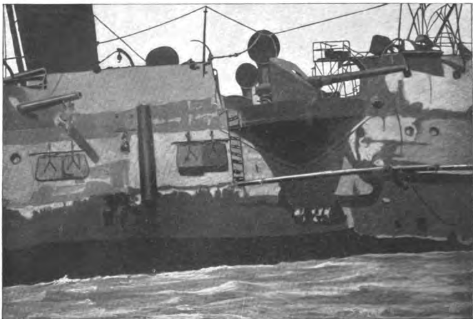
"OQUENDO," STARBOARD SIDE, SHOWING EXIT OF 13-INCH SHELL.
