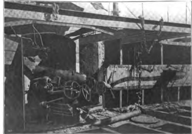
5.5-INCH GUN AND CARTRIDGE ON "VIZCAYA."
