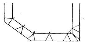
At 2 is at present a platform and embrasure for a field gun. By coupéing it and cutting the embrasures, as represented by the dotted line, a fifth gun might be put here; but, while it might be well to arrange the place for it, I would only place four guns (1, 2, 3, and 4), leaving two in the exterior battery. On the western face I would arrange platforms for four field guns (1, 2, 3, and 4). Embrasares' flare, 60 degrees; platforms, 12 feet wide.
