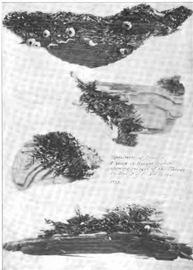
SPECIMEN OF PINE PILE, TWO YEARS IN HABANA HARBOR, SHOWING RAVAGES OF THE TEREDO.
